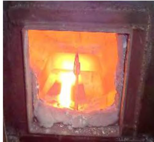
One of the prime questions to be answered by the experiment was whether the coating was tough enough to withstand the repeated handling necessary to heat-cycling the blade. As you can see here, the coating seems to be holding up just fine. The "black" area at the tip of the tang is the bare spot left by the jaws of the vise grips. It gets the usual three times to critical and air cool to black, then to critical a fourth time before quenching.
