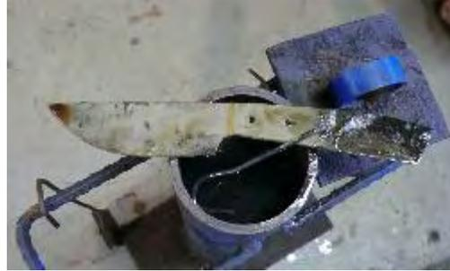
After cooling the blade and wire brushing off the coating, this is what we got. There is little to no evidence of scaling. Hardness is somewhere north of 55 Rockwell C (based on a set of testing files) but under 60, so it is a little softer than it could be, but it is still in an acceptable range.
