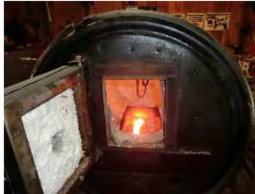
A high temperature probe is inserted through the probe port which places the probe on level with the blade hangers (approximately central in the drum). The probe is a Type-K electrode talking to an Omega hand-held digital pyrometer. As seen here, the temperature is getting close to what is needed.
