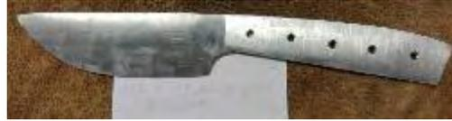
Since the critical temperature (~1550 F) is well in the scaling range, you can expect scale unless you are using a noble gas atmosphere or hot salt. Since we are not, what we will use is a coating that keeps the oxygen off the blade. The first step is to thoroughly degrease the steel (any decent greaser like the ones shown here will suffice). Wash it until water sheets off the blade and then keep those grubby mitts off it there after.
