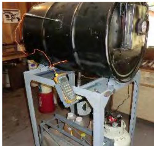
Because of the use of a venturi burner (as opposed to Don's design which uses a blown system), a tiny blower is needed. Without the blower, the pressure in the forge is sufficient to choke the burner. The blower is a 12V squirrel cage and plugs into the bell of the burner. The system needs only 3 to 5 psi to hover at 1550 F and reaches that temperature in about 15 minutes from light off.
